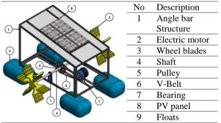
Figure 1. Design of shrimp pond wheels using solar power
